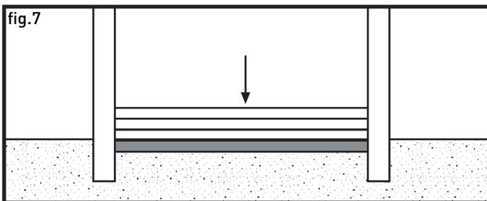
Secure the post as above, and finally, slot the fence panel between the two posts. If required, cut the posts down to size using standard cutting tools and complete by fitting decorative caps to posts.
