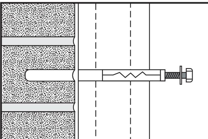
Anchors should be spaced no more than 2ft (0.6m) apart with no less than two in total. Drill the holes in the post first and allow only a small clearance over the shank diameter of the anchor bolt. Offer the post to the wall ensuring it is level in both vertical planes and aligned correctly (using a spirit level and engineers square). If necessary use packing between the post and the wall. Bolt the post firmly into position.
