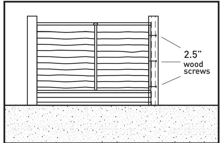
If the first post is in open ground it will again need to be upright and perpendicular to the ground in both vertical planes and facing accurately in the correct direction. Mount in concrete as detailed below then attach to the first fence panel using 2.5" wood screws.
