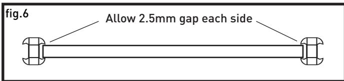
Place the gravel board into the 'H' slot of the post and align. The gravelboard may be sunk into the ground to provide a more secure fitting. Position your next post in place allowing a 2.5mm expansion gap at both ends of the gravelboard (use spacers).
