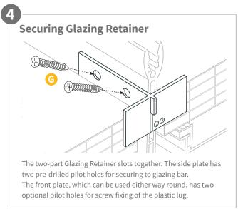
Kit Includes: Glazing Retainer (D), End Cap Lug (E), End Cap (F), 2 x Self-Drilling Screws (G), Standard Screw (H).
