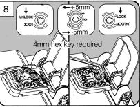
To adjust lateral position, first turn the unlock screw a 1/4 turn. Then use the adjustment screw to adjust up to 5mm in either direction. Finally
