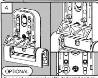
If required an optional profile dedicated packer can be fitted. Align pegs with holes in hinge and push to insert for positive fit.
