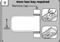
Height adjustment: Using a 4mm hex key turn the screw down to lift the hinge by up to 5mm.
