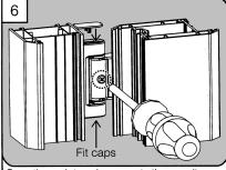
Open the sash to gain access to the security screw location and using screw provided fix in place to secure cover and hinge pin.
