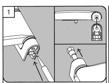
As default the hinge will be set as right handed. To change first ensure that sash part is at a right angle to frame part and push out the pin from bottom. Then reverse sash and refit pin.
