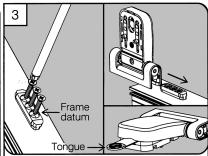
Fit the frame datum into the drilled 5mm holes and screw in place. Take hinge and align the aperture in the frame part and slide into position. Lift sash cover and remove tongue.
